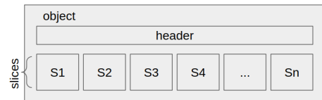
Figure 4: Data object structure
